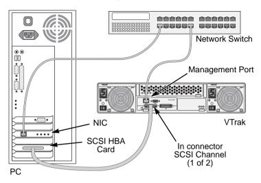
Figure 12. VTrak M300p and M200p DAS connections (M500p is similar)
